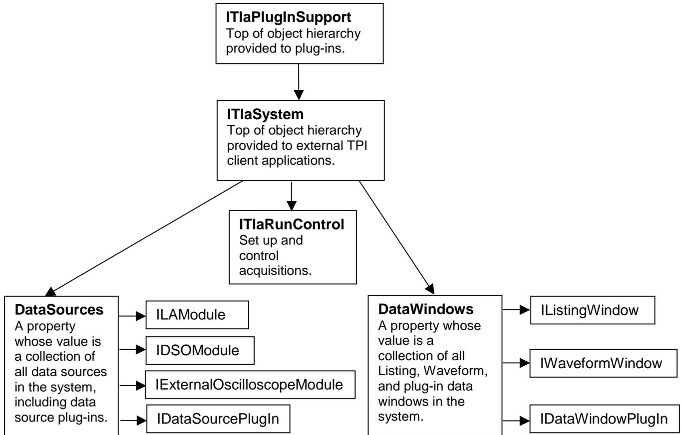
Both plug-ins and remote TPI clients programmatically access the TLA through an `ITlaSystem` object, which maintains collections of all the other objects that make up the system such as data sources and data windows.
