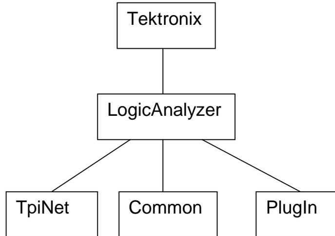
For example the ITlaSystem interface (described in section 2.2) is contained within the TpiNet namespace. Its fully qualified named in the C# programming language is Tektronix.LogicAnalyzer.TpiNet.ITlaSystem.
